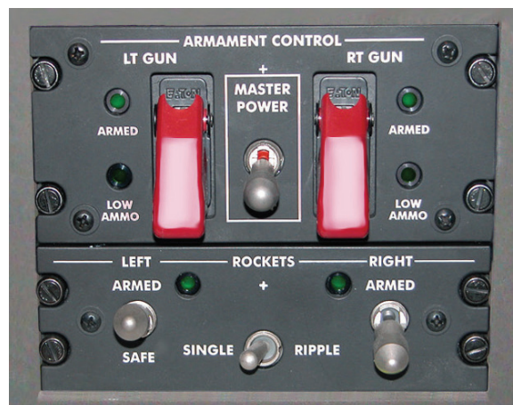
Pilot control box and rocket control panel
