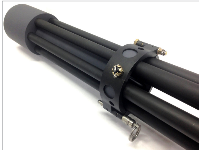
Barrel Clamp Retainer Assembly, installed
