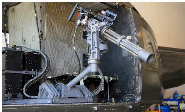
Kick-out weapon mount with an M134D deployed
