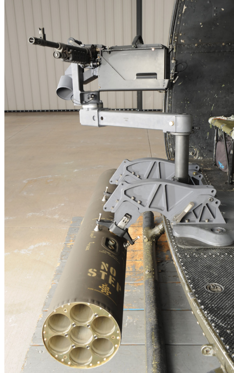
Outboard station with an M260 rocket pod (also showing the mount with an M240/MAG58)
