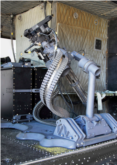
Kick-out weapon mount with an M134D retracted
