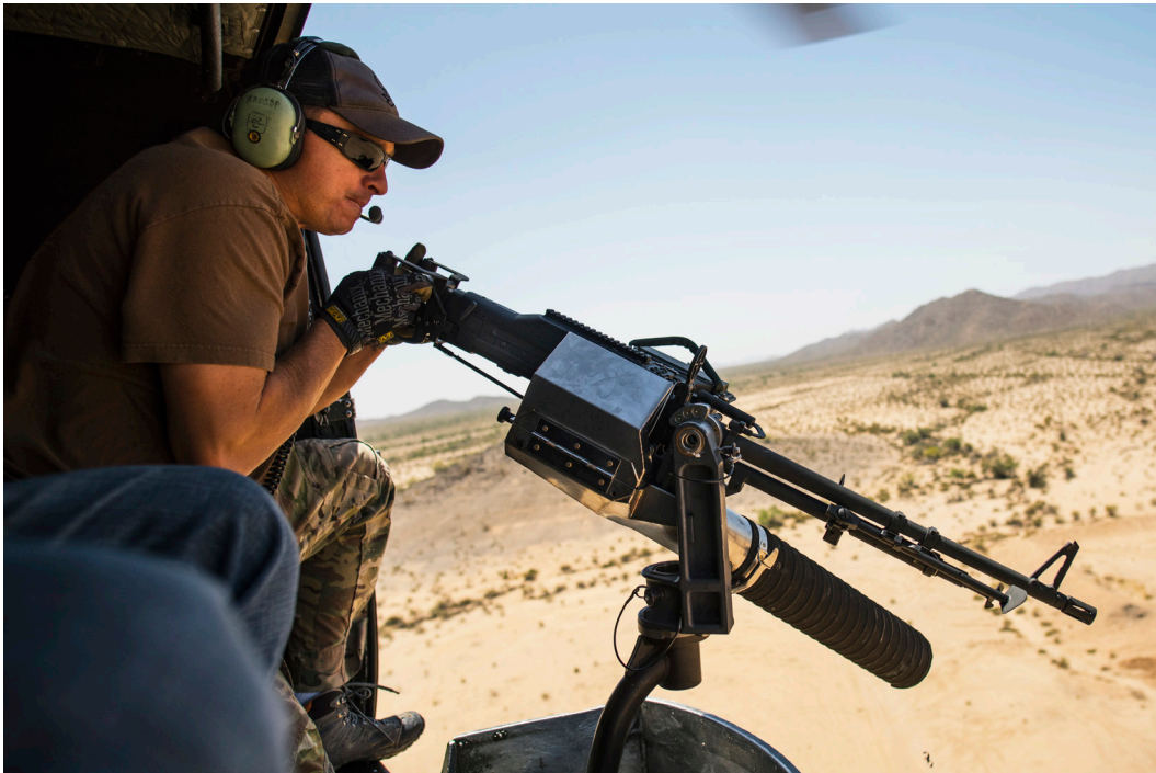
M60 Mount in-flight on a UH-1 helicopter
