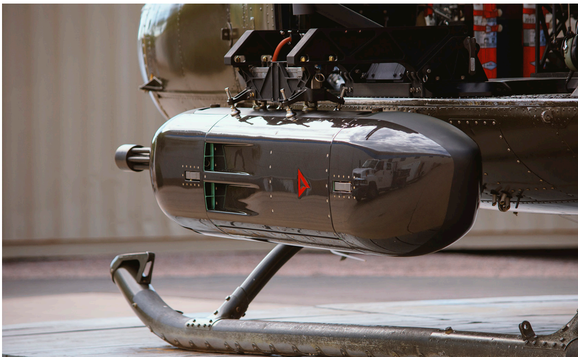
UH-1 equipped with DAP-6 Gun Pod
