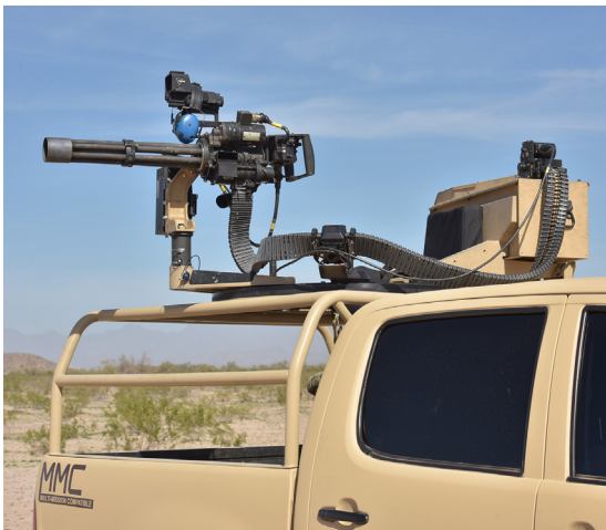
Dillon Aero MMC Vehicle System with a 3,000-round magazine for ground applications
