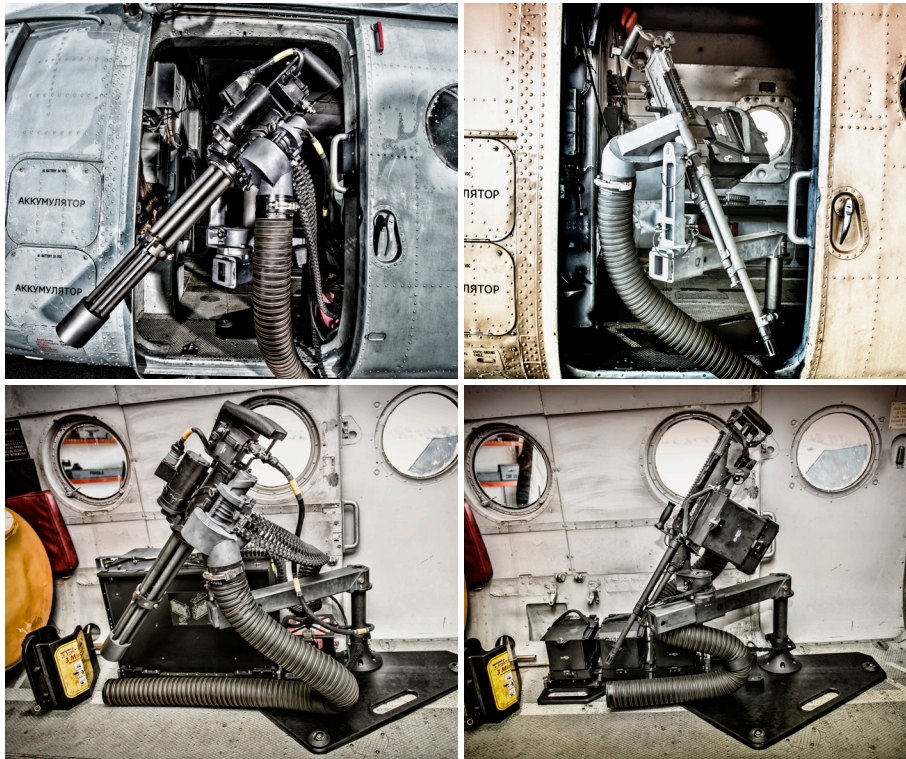
Dillon Aero Mi-17 Mount armed with a PKM, M240/MAG58/GPMG, and the M134D minigun
