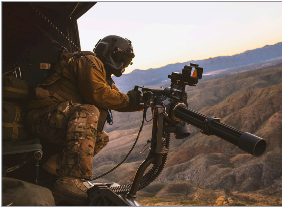
Dillon Aero Huey Mount armed with M134D Minigun
