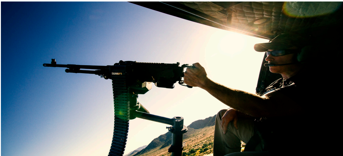
M240/MAG58 Mount in-flight on a UH-1 helicopter
