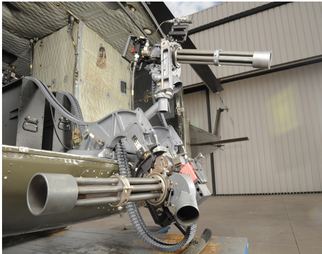
Left side stations with Fixed Forward and Crew-Served M134D-H miniguns
