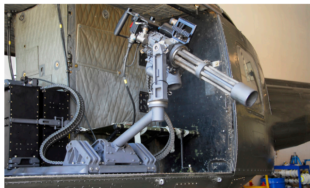
Kick-out weapon mount with an M134D deployed
