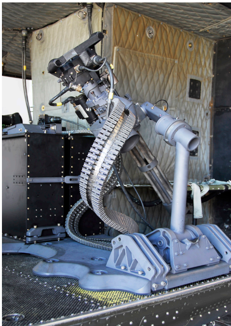
Kick-out weapon mount with an M134D retracted
