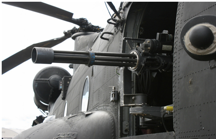
Chinook helicopter affixed with the Chinook Mount and M134D Minigun
