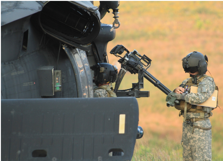
Black Hawk Window Mount with M134D installed
