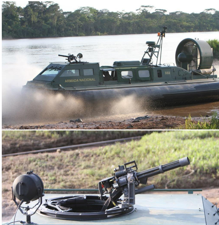
A Griffon Hoverwork hovercraft equipped with the Dillon Hovercraft Mount and M134D gun
