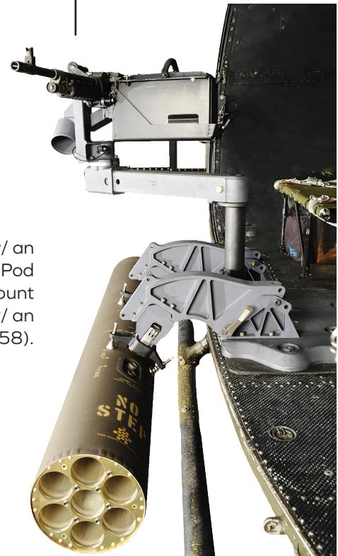
Outboard Station w/ an M260 Rocket Pod (Also shown-Mount with w/ an M240/MAG 58).
